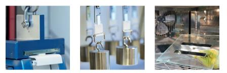
**Exclusive Application Testing:** In its application laboratories, tesa analyzes the customers' materials in combination with several adhesive tape solutions. Depending on the customer-specific demands, the analysis includes test on the resistance to UV-light, high and low temperatures, peel adhesion, shock and tension absorption and much more. The result: adhesive tape solutions perfectly suiting any technical application.
