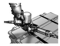
All pneumatic sealers are furnished with a quick-disconnect plug. An air filter and regulator are necessary.
