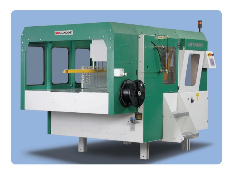
**S**quare and strap bundles automatically, in-line with the Signode ISB strapping system. Signode ISB bundling machines range from the economical single-pusher, single head model to a high-speed dual-head system with independent pushers to strap up to 30 bundles per minute.
