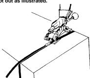
7. Excess strap is bent sharply back on the seal with the thumb or fingers. One and a half or two additional bends will result in a clean strap break off. If the width and gauge of the strap being used will not allow it to be bent, cut the excess strap as close to the seal as possible using an approved strap cutter.
