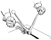
Return the handle to rest on the tool and press down on the handle pawl with thumb. Squeeze the handle to the base and remove the tool from the strap by swinging the rear foot out as illustrated.
