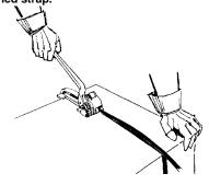
Snap a seal on the straps directly in front of the tool, making sure that the seal covers both straps.
