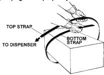
2. Hold the hand-tensioned strap in position with the left hand, grasp the tool in the right hand and squeeze the handle to the base to lift the feedwheel. Position the rear foot over the strap and slide the front foot under the overlapping ends, approximately 1" (25mm) ahead of the lower strap end. Make sure both straps have been fully inserted into the tool. The inner edges of the strap must butt up against the inner edge of the tool.
