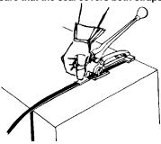
Hold the sealing tool at a right angle to the strap and rest it squarely over the seal. Seal the tensioned strap by bringing both sealer handles together as far as they will go.
