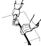
3. Release grip on tool to engage straps. Make sure the strap is in alignment with the tool. While standing to one side of the strap line, tension the strap through continuous up and down motions with the tensioning handle. NOTE: Do not allow the handle to press against the base during the downward portion of the tensioning cycle. This will raise the feedwheel and release the tensioned strap.
