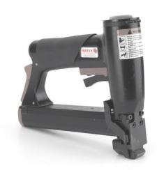
The Dial-a-Flare foam stapler features a contact-trip mechanism that is designed for foam stapling, ensuring quick and easy actuation. This stapler was built for heavy-duty production, delivering the reliability and consistency you need. The single-flare adjustment means less parts and easy bottom-loading means you waste less time reloading. Our tool-steel nose and flare parts are designed for extra durability and resilience.
